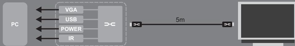
The umbilical connects through a small breakout PCB fitted to an expansion slot in your PC
